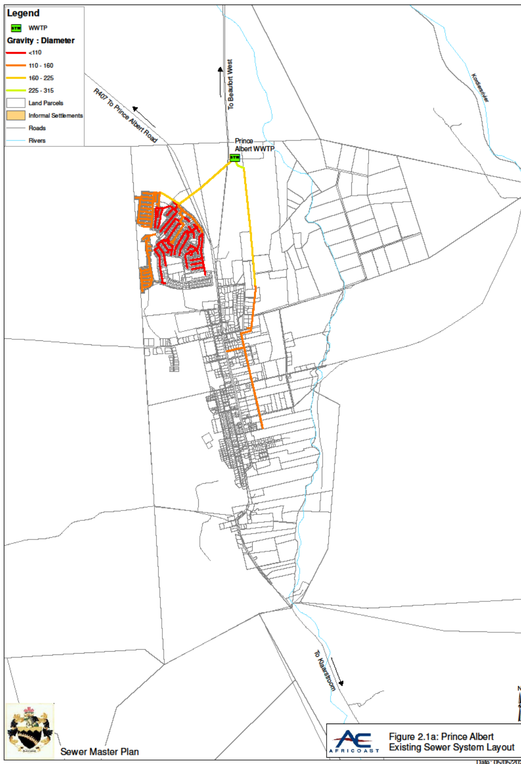
Figure 2.1a: Prince Albert Existing Sewer System Layout
